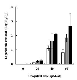
Figure 4. Effect of coagulant dose on rNV-VLP, Q $\beta$ , and MS2 removals after settling in the coagulation process with PACl at pH 6.8. White, gray, and black columns represent rNV-VLPs, Q $\beta$ , and MS2, respectively. Values are means and standard deviation of two or three replications.
