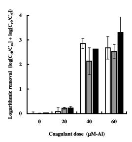
Figure 7. Effect of coagulant dose on rNV-VLP, Q $\beta$ , and MS2 removals in the coagulation–rapid sand filtration process with PACl at pH 6.8. White, gray, and black columns represent rNV-VLPs, Q $\beta$ , and MS2, respectively. Values are means and standard deviation of two or three replications.
