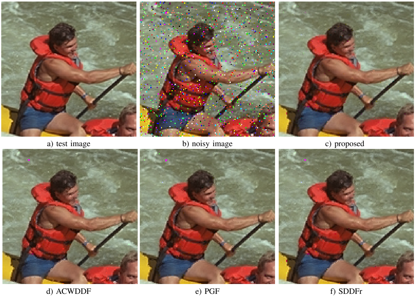
Fig. 13: Comparison of the denoising results obtained with the new filtering technique in comparison with other filtering methods, (test image RAFTING contaminated with uniform noise, p = 0.1 ).
