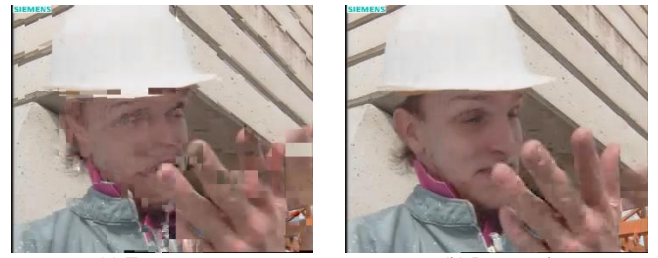
(a) Frame copy (b) Proposed Fig. 6. Comparison of the subjective quality of the 154 th frame on Foreman sequence under 10% packet loss ratio.
