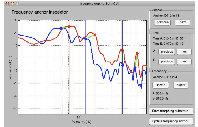
Fig. 15. GUI for frequency anchor assignment. Blue and red lines represent STRAIGHT spectrum slice at anchoring points on example A and example B respectively.
