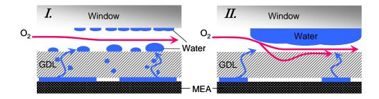
Fig. 13. Experimentally suggested liquid water distribution and gas flow paths: (I) corresponds to the early stage of the gradual voltage drop, and (II) for the stabilized high-voltage stage with large pressure drops.
