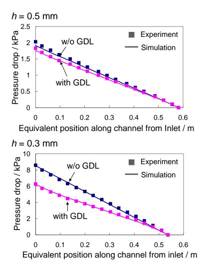
Fig. 7. Comparison between the simulated and experimental results of pressure drops along the serpentine channel for two different channel heights, *h*.
