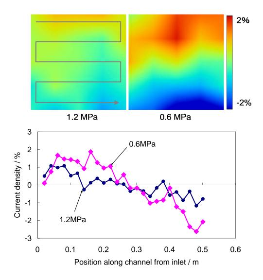
Fig. 9. Current density distributions at two different clamping pressures, 1.2 and 0.6 MPa, for the 1.4 stoichiometric ratio, 240 seconds after the start of experiments.
