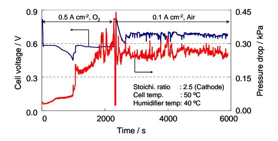
Fig. 14. Cell voltage and pressure drop in the cathode flow for the case with O<sub>2</sub>-air exchanging.
