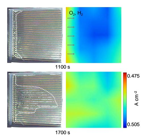
Fig. 12. Current density distribution and direct view in the cathode channel at three different times in the Fig. 11 experiment for the 2.5 stoichiometric ratio.
