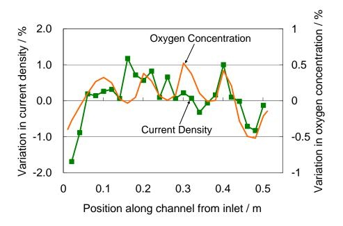
Fig. 10. Variations in the measured current density and the estimated oxygen concentration for the clamping pressure of 0.6 MPa.
