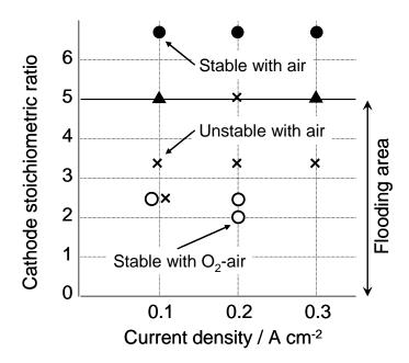
Fig. 15. Stability of operation with air and the case with O<sub>2</sub>-air exchanging.
