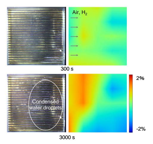
Fig. 4. Direct view in the cathode straight channel and current density distribution at two different times in the Fig. 2 experiment for the 2.0 stoichiometric ratio.
