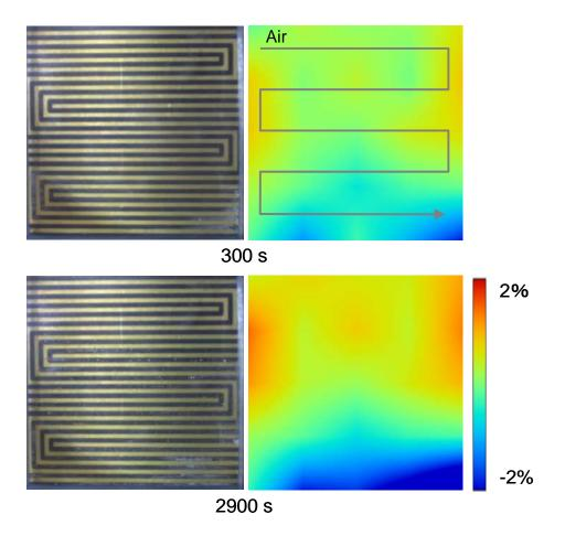
Fig. 5. Direct view in the cathode serpentine channel and current density distribution at two different times in the Fig. 3 experiment for the 2.0 stoichiometric ratio.
