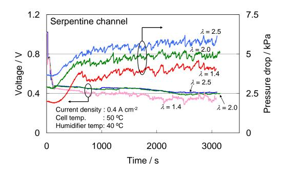
Fig. 3. Cell voltage and pressure drops in the cathode flow for three different stoichiometric ratios of air,  $\lambda = 1.4$ , 2.0 and 2.5, in the serpentine channel.
