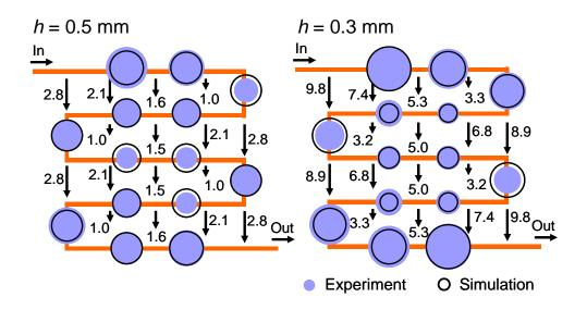
Fig. 8. Flow rate distributions through channel, expressed in circle size, and GDL under the lands, which is expressed in percentage of the total flow rate. The conditions correspond to the cases with GDL in Fig. 7 for two different channel heights, *h*.
