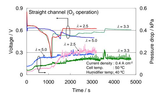
Fig. 11. Cell voltage and pressure drops in the cathode flow in the flooded conditions for three different stoichiometric ratios of oxygen,  $\lambda = 2.5$ , 3.3 and 5.0, in the straight channel.
