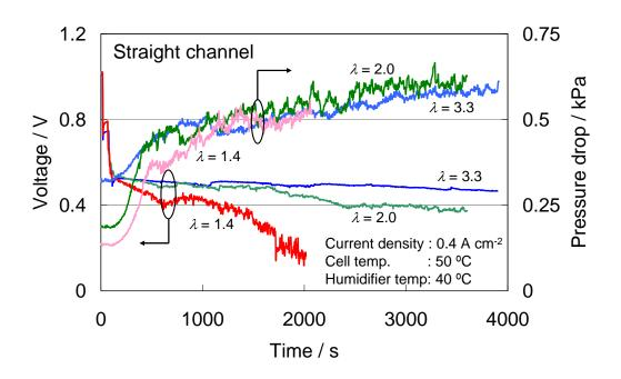
Fig. 2. Cell voltage and pressure drops in the cathode flow for three different stoichiometric ratios of air,  $\lambda = 1.4$ , 2.0 and 3.3, in the straight channel.
