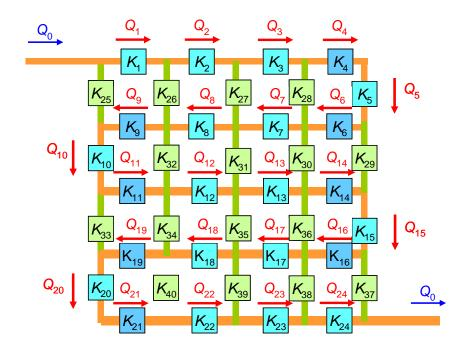
Fig. 6. Simple circuit model of the gas flow in the serpentine separator channel.
