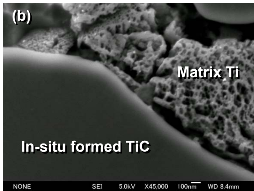
Figure 4: Optical microstructure of P/M extruded TMC with CNTs (a) and interface observation between TiC and titanium matrix (b) observed by scanning electron microscopy.
