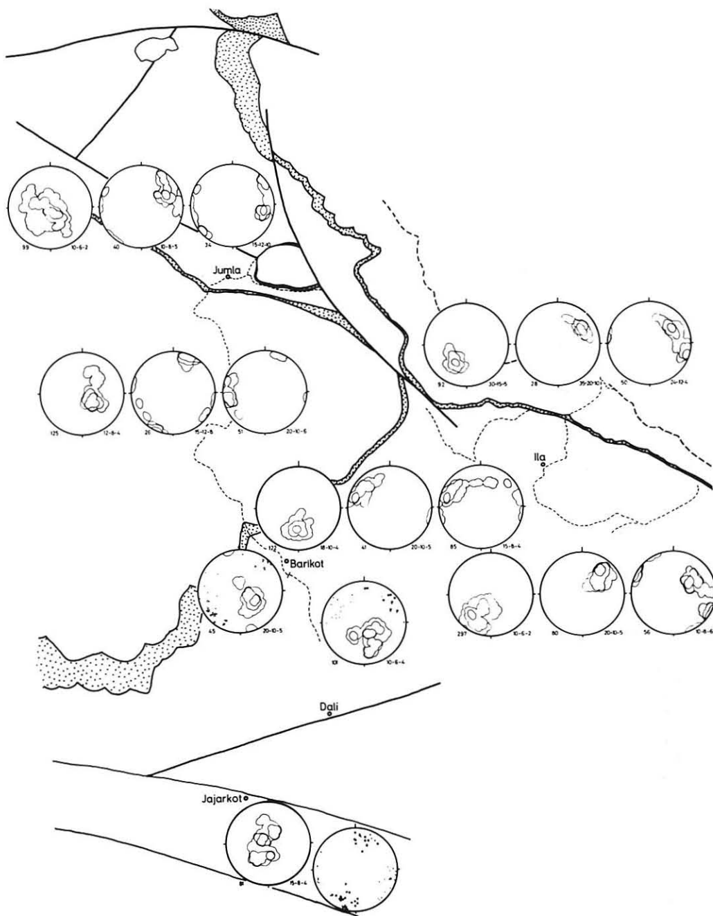
Text-fig. 5 Fabric diagrams showing bedding and foliation planes, mineral lineation and axis of micro-folding. Three diagrams in a row represent bedding or foliation planes, mineral lineation and axis of micro-folding from left to right. In single diagram contours, open circles and solid circles represent bedding or foliation planes, mineral lineation and axis of micro-folding, respectively. The figures at bottom left and right of each diagram are the number of element measured and the percentage number of the contours, respectively. Projected on lower hemisphere.
