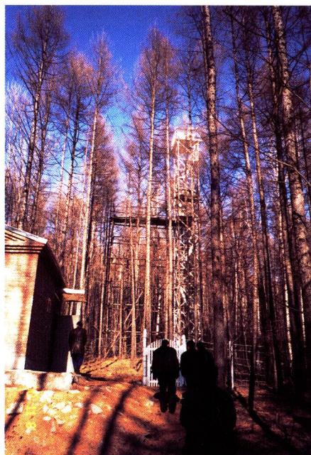
Photo. 7. A view of CO 2 flux monitoring tower (height 24m plus a 3m pole for setting CO 2 monitoring) Left: Field laboratory for operating CO 2 analyzers with air conditioner.
