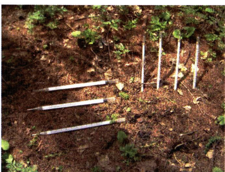
Photo. 6. Setting pF meters for measuring soil moisture condition
