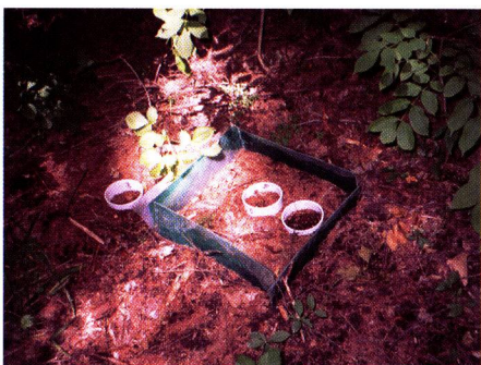
Photo. 5. Measurement of soil respiration with trenching method. White cycles are holders of a chamber for respiration measurement.
