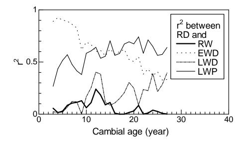
Fig. 5. Trends for coefficients of determination  $(r^2)$  between RD and RW, EWD, LWD, and LWP associated with cambial age
