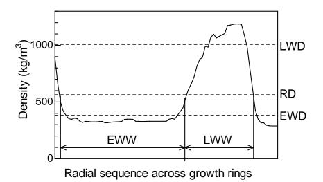
Fig. 2. Definition of growth ring parameters obtained by X-ray densitometry LWD: Latewood density, RD: Average wood density within a ring, EWD: Earlywood density, RW: Ring width (EWW+LWW), LWP: Latewood percentage (LWW/RW  $\times$  100) Threshold density (boundary between earlywood and latewood): 550kg/m<sup>3</sup>
