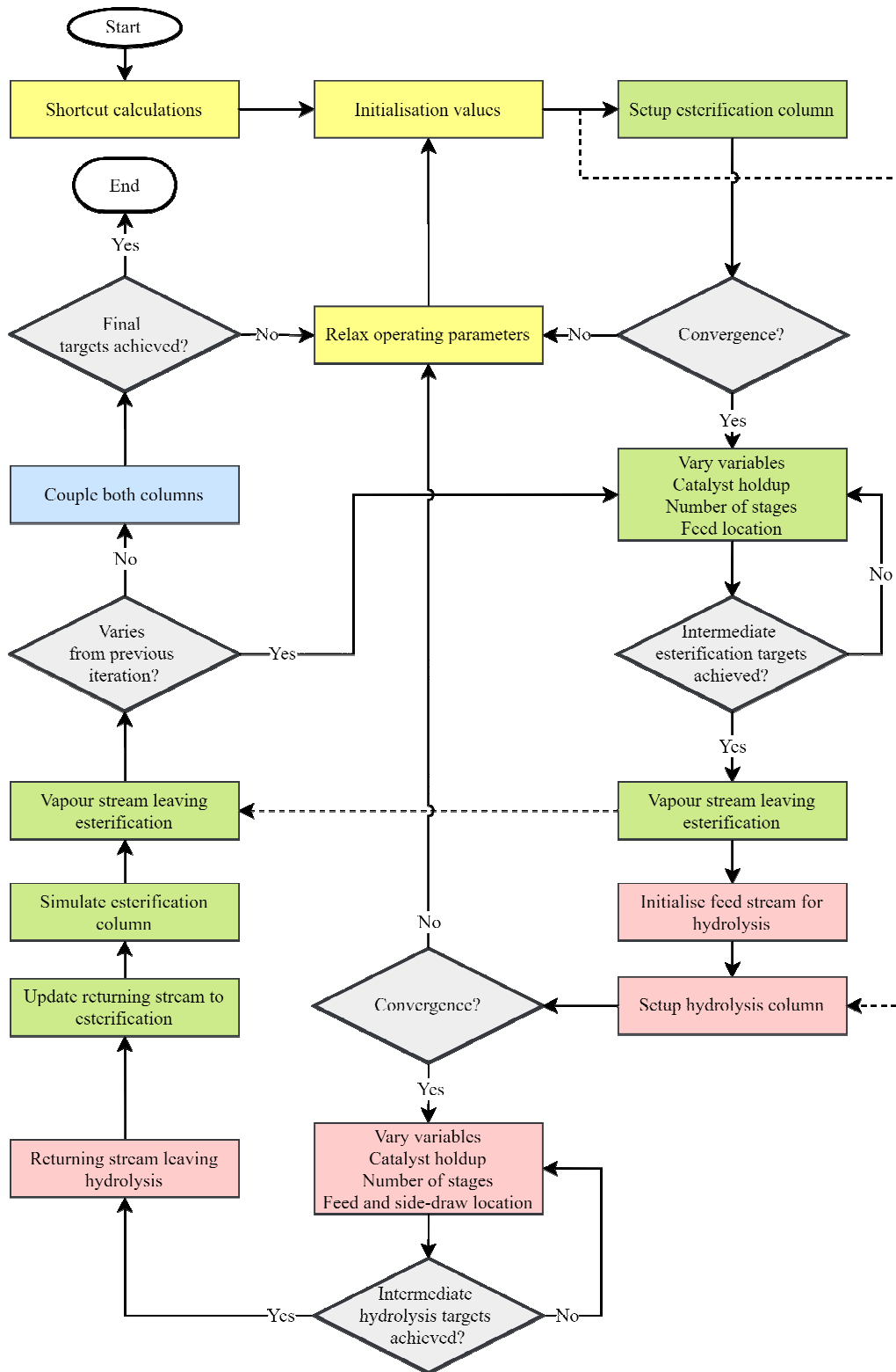
Figure 3. Methodology to implement a rigorous simulation of a fully-thermally coupled arrangement with two reactive sections (dashed connections considered after first iteration, yellow: initialisation values adjustment, green: esterification column implementation, red: hydrolysis column implementation, blue: coupling)
