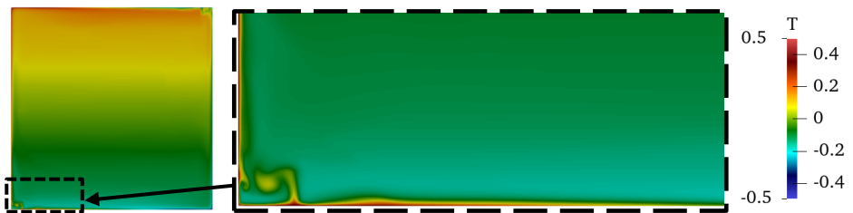
Fig. C.6. An instantaneous snapshot of the RANS temperature from a hybrid simulation in which the LES zone
