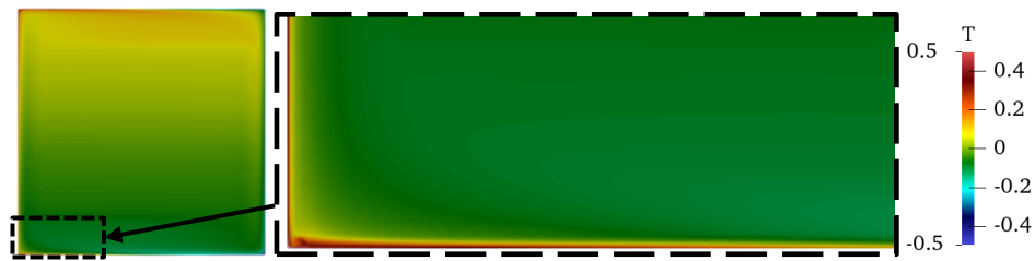
522 Fig. 15. An instantaneous snapshot of the RANS temperature from a hybrid simulation in which the LES zone 523 weight was calculated using Equation (44). A zoomed-in view of the contours near the bottom left corner is 524 provided as well.
