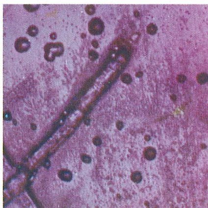
Photo, 12 Rimed droplets on an ice surface at -10^{\circ}\text{C} . \times 104
