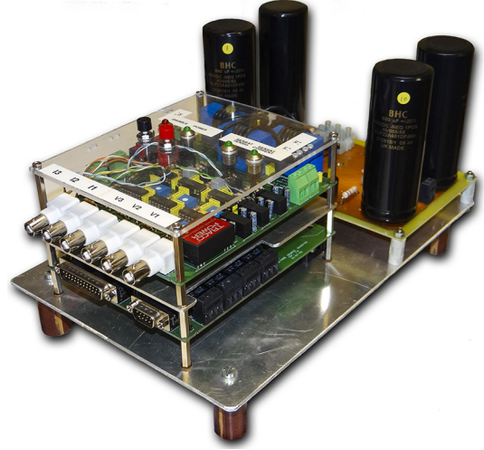
Figure 1. Prototype of the boost converter employed for the experimental analysis of the efficiency models.
