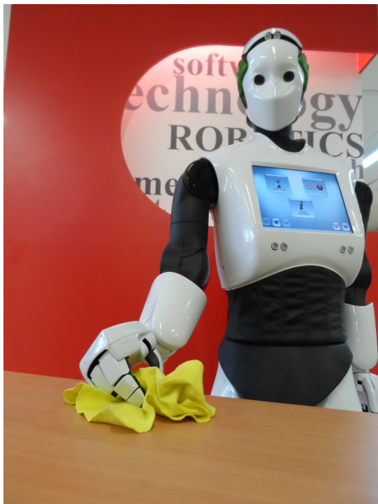
Fig. 5. The REEM robot grasping a textile. Textiles and other deformable objects are common in everyday environments, but still not considered in competitions as deformable object manipulation is challenging.
