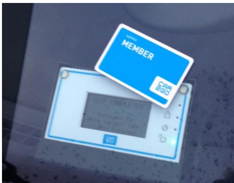
Figure 4.2: Member card and NFC sensor that opens the car
