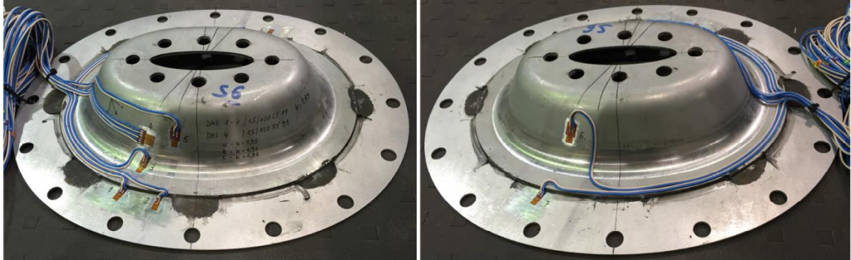
Figure 5-8: Location of the strain gauges on cup-shaped specimens
