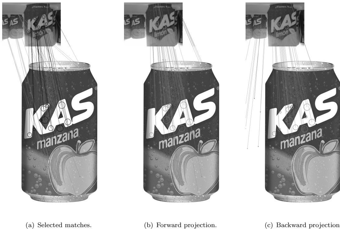
FIGURE 6.10: Retrieval example with many instances of one object present in the query scene. Query images are displayed above reference images. Projections are done according to the best found transformation model. (a) Selected matches. Inliers and outliers are represented with black and grey colours respectively. (b) Projection of reference key-points into query image. (c) Backward projection of query key-points into reference image.
