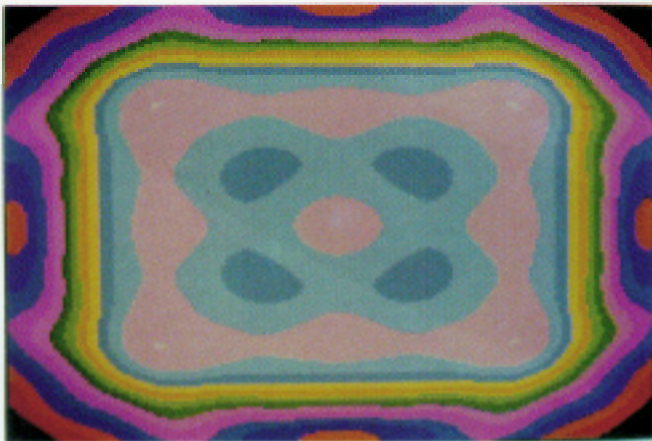
Fig. 7. Square object composed with fat, muscle, and bone surrounded by water. Reconstruction (modulus of \hat{K}(x, y) ) displayed on a TV monitor.
