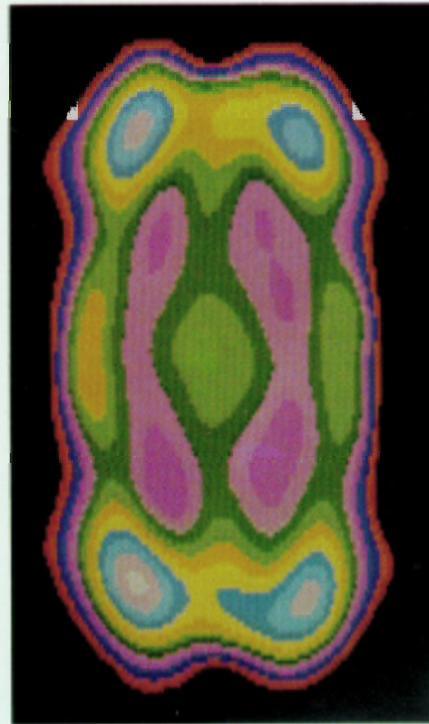
Fig. 8. Section of simulated human arm (upper segment) surrounded by water. Reconstruction (modulus of \hat{K}(x, y) ).
