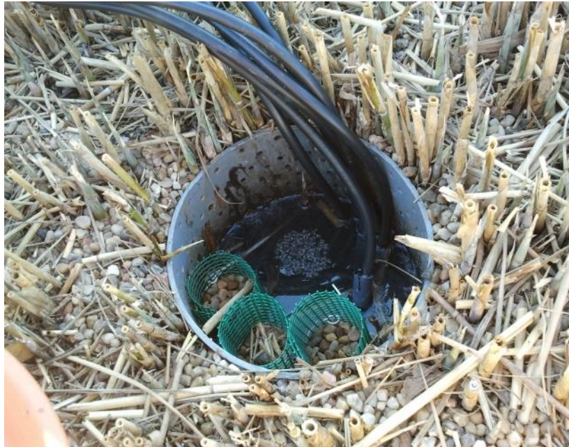
2 Figure 1. Microbial fuel cells implemented within the wetland at the beginning of the 3 experiment.
