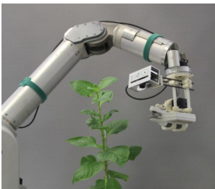
Figure 4. Setup used to take chlorophyll measures from suitable plant leaves, with the Barrett WAM arm carrying a time-of-flight camera and a spad meter. Observe that the leaf-probing task requires clearance (above and below) of a segment in the border of the chosen leaf.
