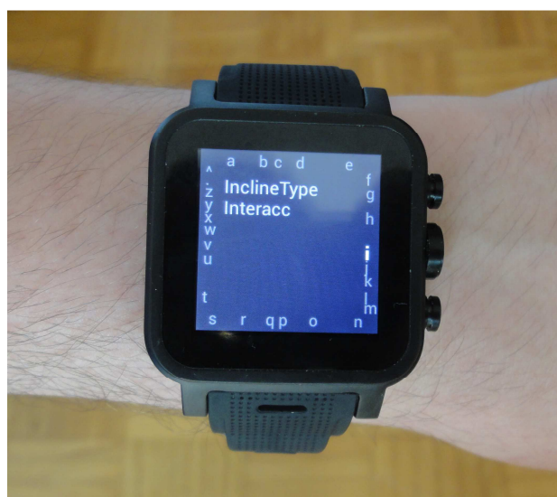
Figure 1: Typing by inclination of smartwatch.
