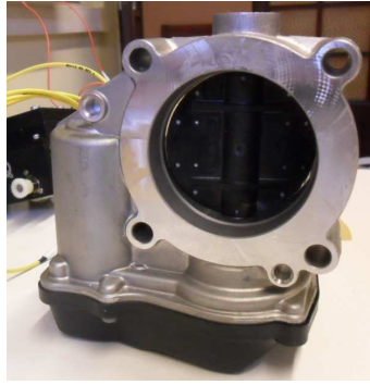
Figure 1. Automotive electronic throttle device used in the experiments described in Section 3.
