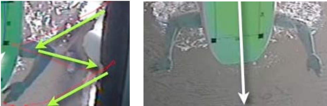
Figure 9. Description of a lateral sculling experiments, measuring propulsion only due to sculling on top of a floating board, air bubbles were also injected to visualize the wakes
