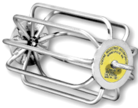
Figure 1. Steel Deflection Gauge - Mandrel Test.
