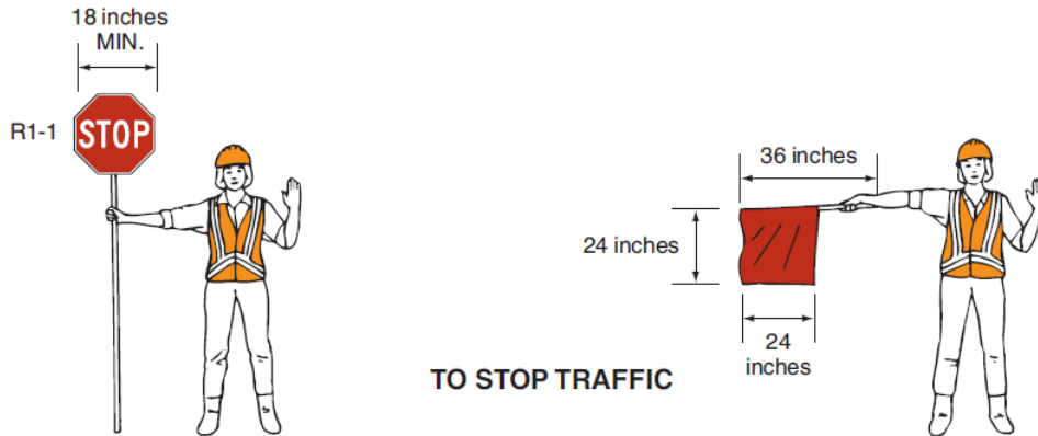
Figure 4. Typical Flagging operation to stop traffic.
