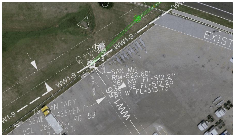
Figure 5. Detail - Initial manhole FL elevations.
