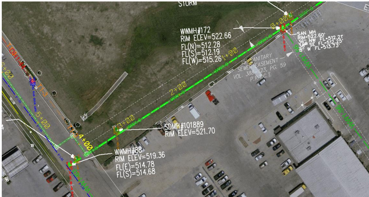
Figure 8. Detail - Lateral connection at Pharr street.
