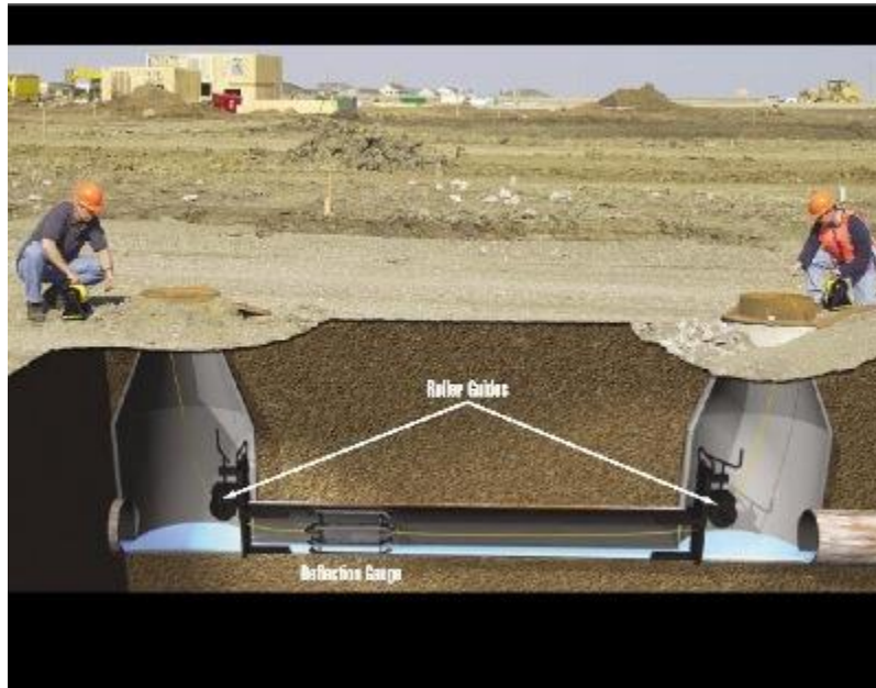
Figure 2. Test Execution - Mandrel Test.
