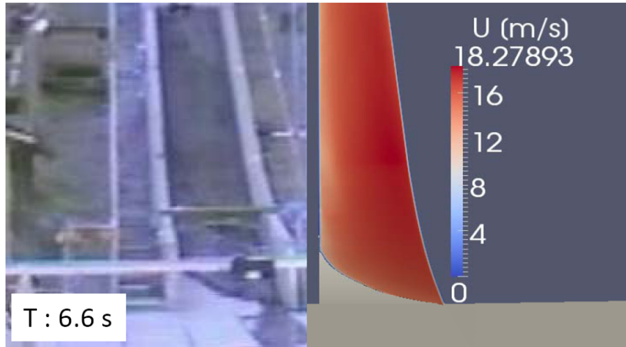
Figure 6. Observed and simulated flow front at the end of the channel for a smooth channel bed and high content of loam. The free model parameter \tau_{00} was calibrated to 90 Pa to gain an identical arrival time in experiment and simulation. The simulated time was measured from the moment of release and the corresponding experimental time was derived by counting the number of video frames in the overview camera video between release and arrival in the run-out plane.
