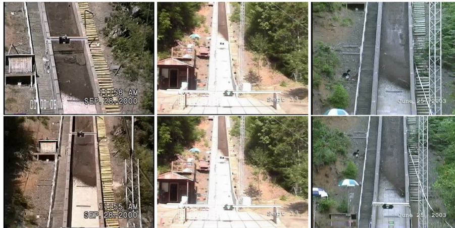
Figure 11. Snapshots of the flow front of test 000928 (left) 5.6 s after release (bottom left) when the approaching second surge (top left) unified with the front. The same happened in test 010913 (center) 7.4 s after release (center bottom) and in test 030625 (right) 7.0 s after release (right bottom). The upper pictures were taken about half a second earlier in time than the lower row. The times of unification shown in the lower row coincided with a sudden increase in front velocity, see Fig. 10 .
