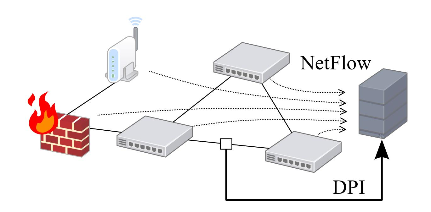
NetFlow as main data input. Auxiliary DPI input to train the application clasification engine, which is applied to *all* the traffic.
