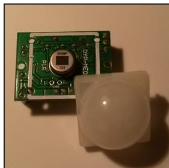
Fig. 7.29 – PIR sensor module with detached diffuser.
