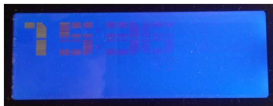
Fig. 7.12 – Flicker cause by calling the clear() method too often (at every loop).
