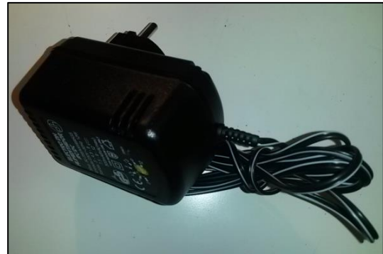
Fig. 7.9 - Power supply with selectable output voltage.
