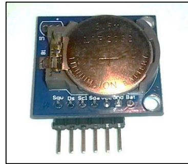
Fig. 7.26 - ds1307 Real Time Clock module.
