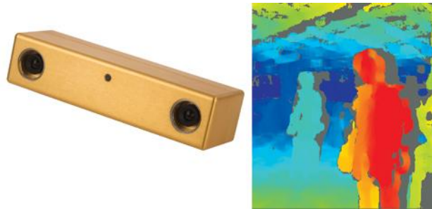
Figure 14. Stereo imaging camera (right side) and depth map (left side)
