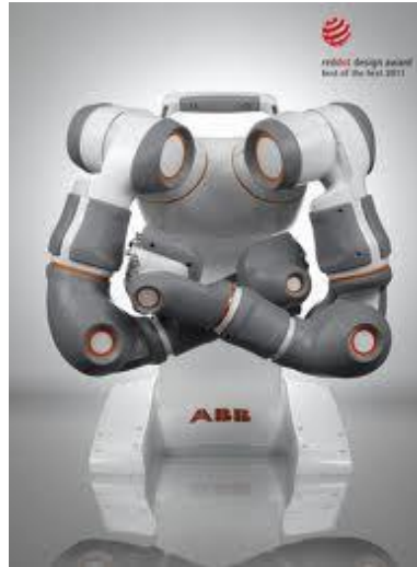
Figure 4. A flexible dual arm for small assembly (Yumi from ABB)
