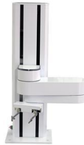
Figure 7. The first collaborative scara robot (pf 400 from precise automation)
