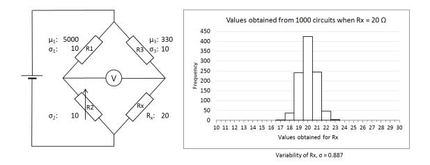
Figure 4: Values obtained for a resistor of  $20 \Omega$  for 1000 circuits with the indicated
