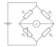
Figure 1: Diagram of a Wheatstone Bridge
