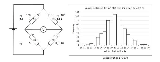
Figure 2: Values obtained for a resistor of  $20 \Omega$  in 1000 circuits with the indicated characteristics
