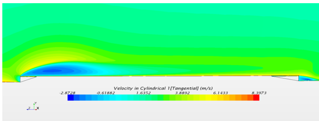
Fig 26. Velocity contour plot. Disk with roughness 1
