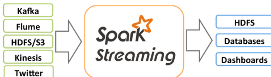
Figure 2.7: Spark streaming diagram. There are many ways to insert data to Spark streaming, like Kafka 13 , Flume 14 , HDFS, etc. Once this data is processed can be saved in HDFS, databases and dashboards. 15
