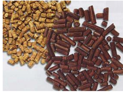
Picture 2.6.5. Different types of pellets for use as fuel in a biomass boiler.
