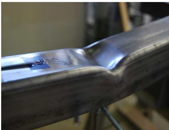
a) Three-point bending loading conditions (no wooden blocks)
