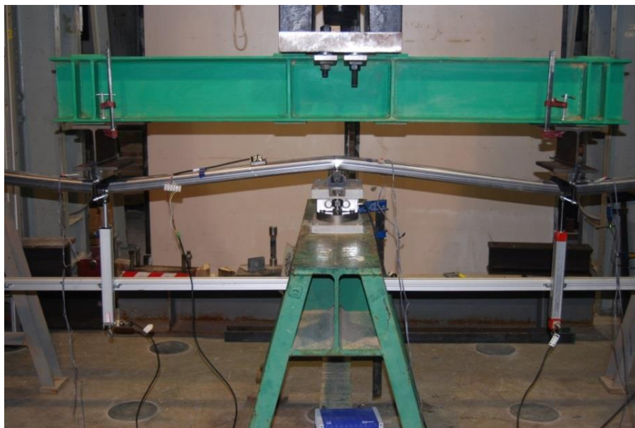
Figure 9. View of the central failed section for the S3-Mi-5P specimen.
