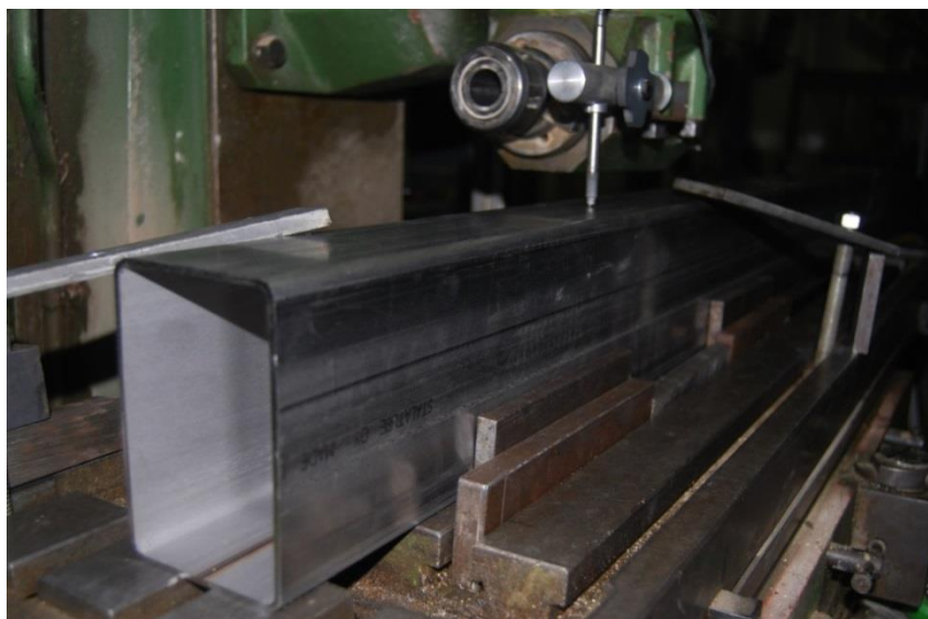
Figure 2. Local imperfection measurement for the S4-Mj-4P specimen.
