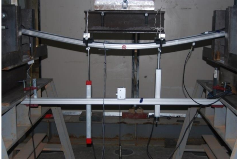
Figure 6. General view of the S3-Mi-4P test under four-point bending conditions.
