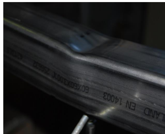
b) Four-point bending loading conditions (wooden blocks)
