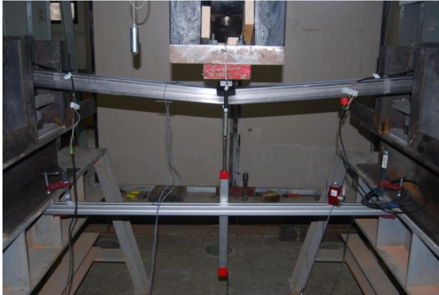
Figure 3. General view of the S2-3P test under three-point bending conditions.
