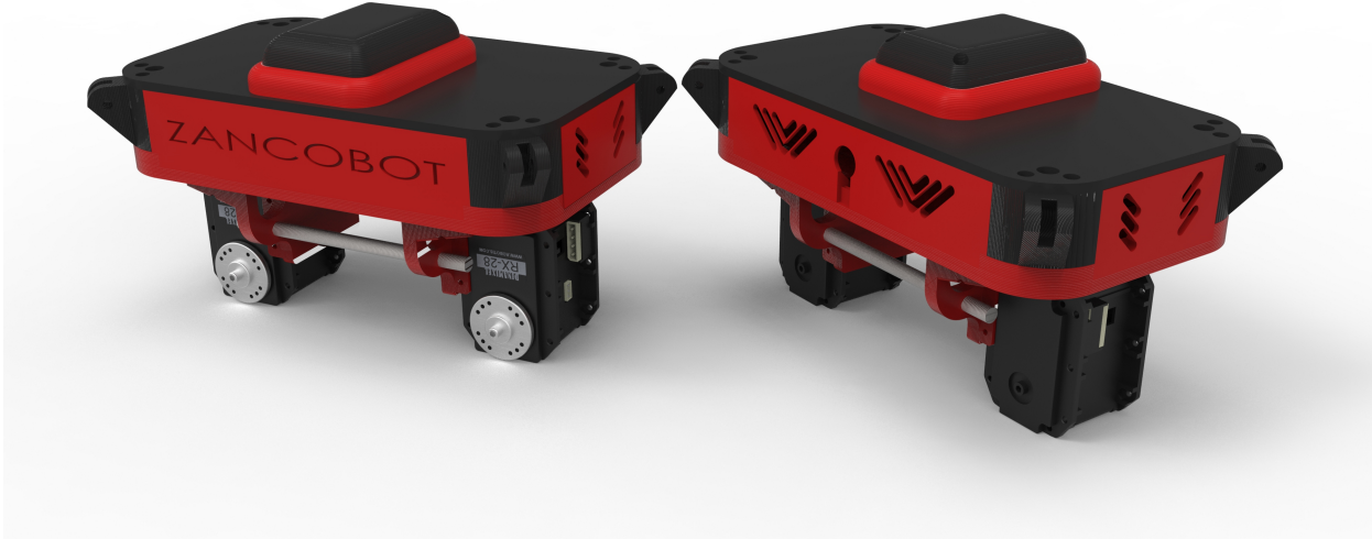
Figure 4.5.1: Chassis of the slim version.
