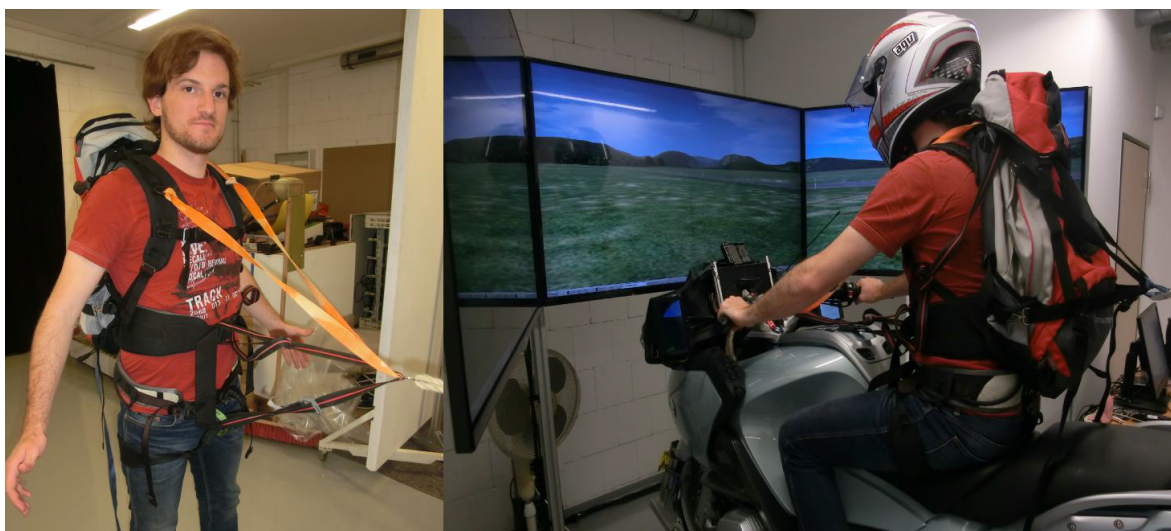
Figure 4-1.: Left part: System consisting of a backpack and a climbing harness. It is set of the braking configuration. Right part: The system during the simulation. (Hanselka, 2014)
