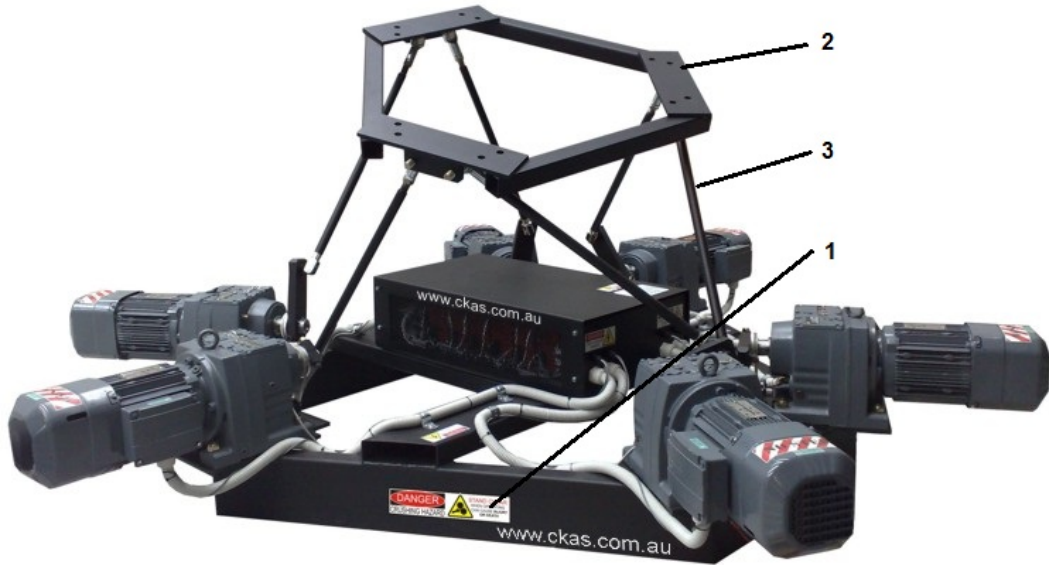
Figure 2-5.: Hexapod: a 6 DOF Motion Platform (1 base, 2 top plate, 3 actuators) (Ckas, 2015)
