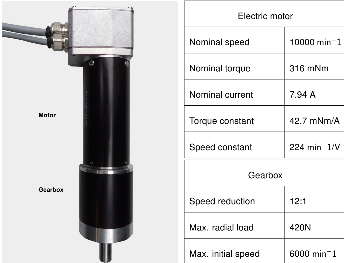
Figure 4-4.: Electric motor with planetary gearbox Table 4-1.: Characteristics of motor and gearbox
