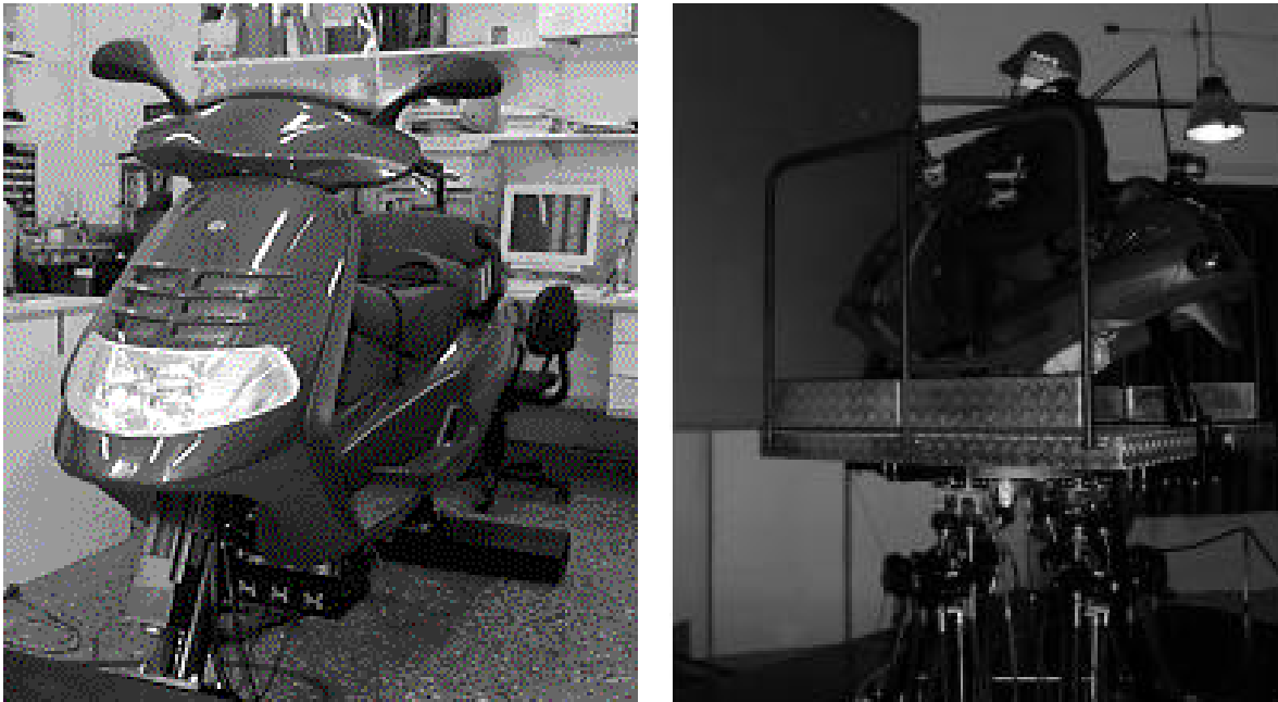
Figure 2-13.: Left part: Mock-up subsystem. Right part: Integrated simulator (Ferrazzin et al., 2001)
