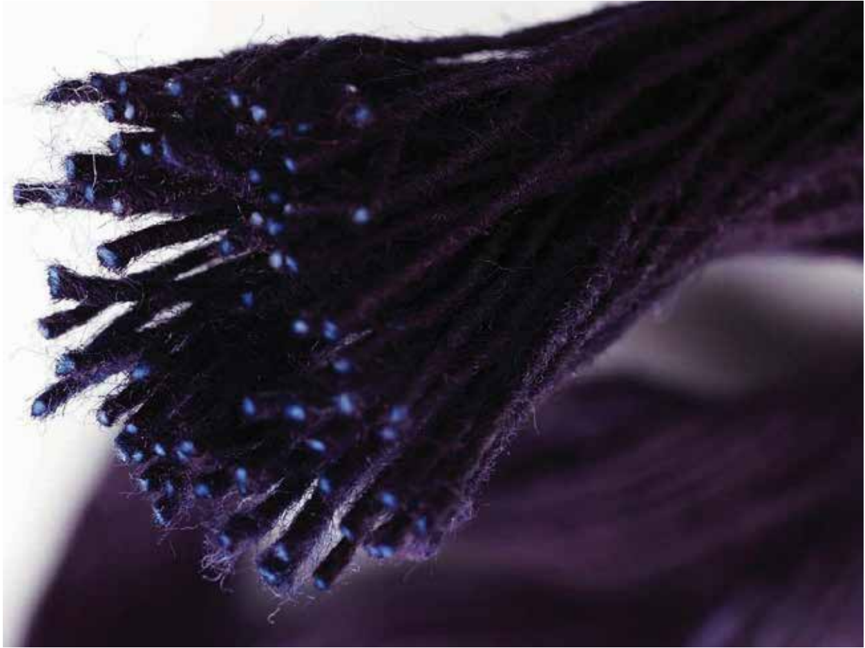
Denim fabric after a bottoming-type application. The initial dyeing performed with a sulfur dye and later with indigo
