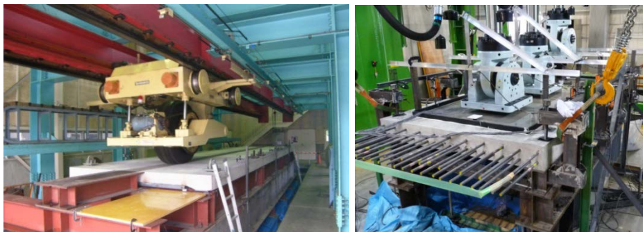
Figure 9: simulated RC bridge slab [18]
