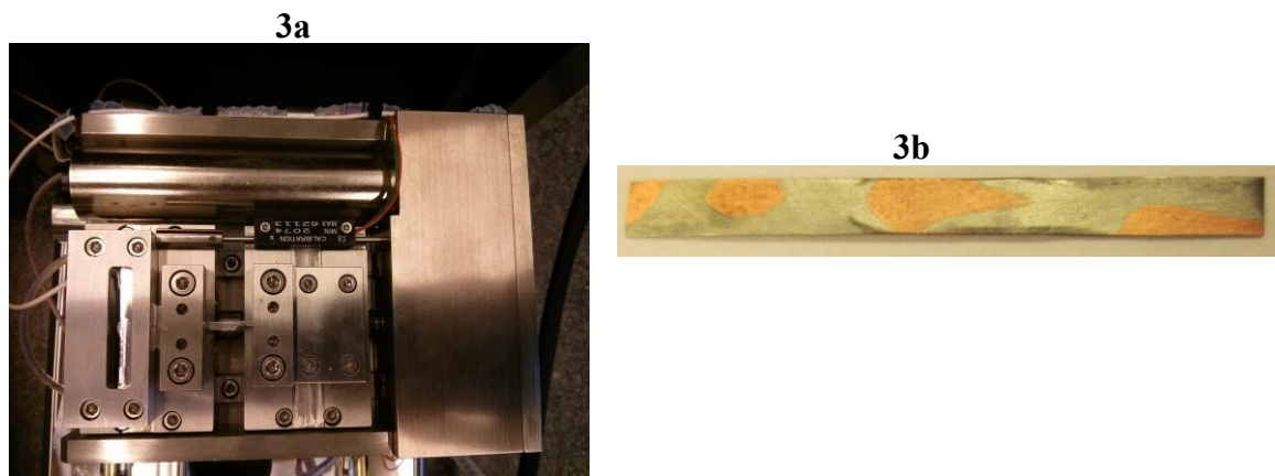
Figure 3: a) tensile stage b) a busbar partially etched to show its bi-material composition.
