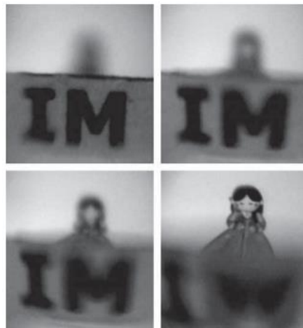
Figure 16 Images that that prove what EW based fluid lens are capable. The letters 'IM' are situated closer to the lens than the doll. When the voltage applied is changed, the focal plane is moved from near to far, and this way the letters 'IM' and the doll are sequentially focalized (Taken from Kang et al. 108 )
