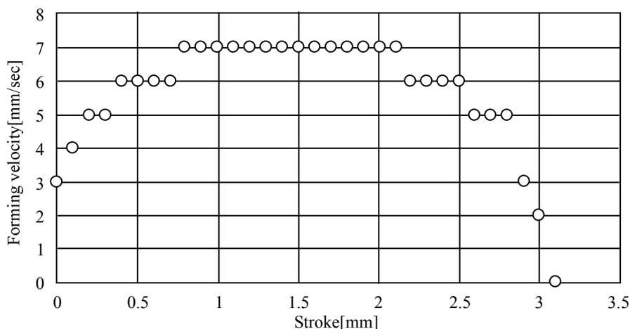
Figure 2: Relationship between forming velocity and stroke
