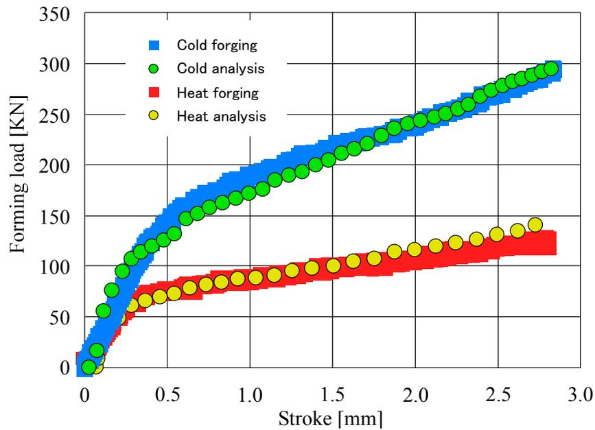
**Figure 3:** Relationship between forming load and stroke
