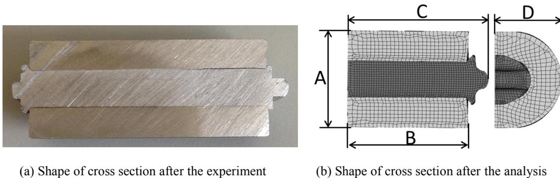
(a) Shape of cross section after the experiment
