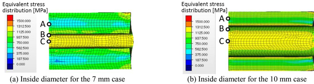
**Figure 13:** Equivalent stress distribution of stainless steel with the stainless steel pipe used as the blank
