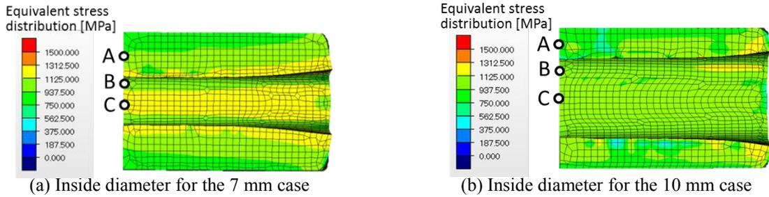
**Figure 12:** Equivalent stress distribution of stainless steel with the two-metal blank
