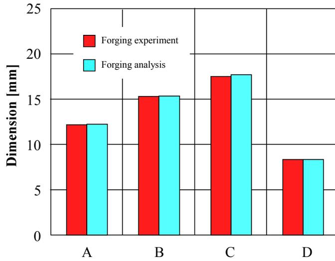
Figure 5: Dimensions of cross section shape after forming
