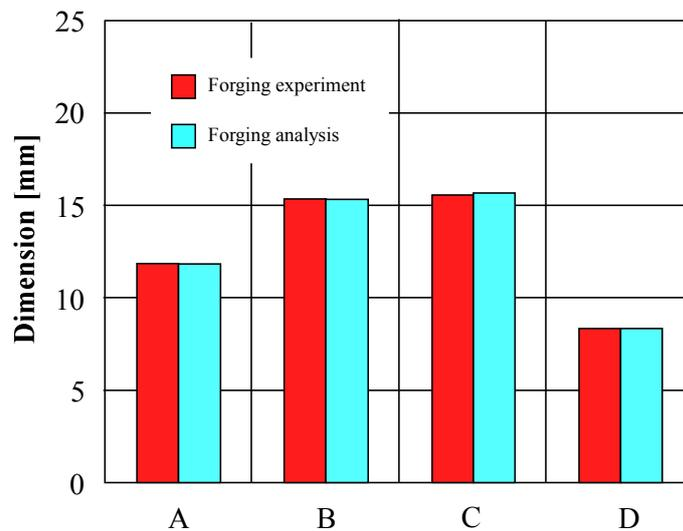
Figure 7: Dimension of cross section shape after cold forming
