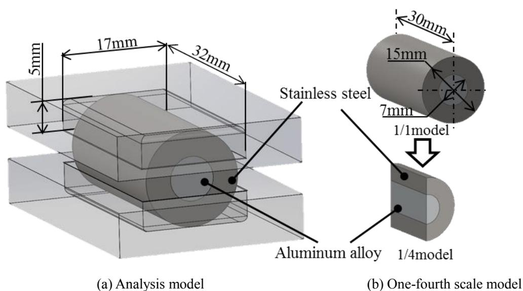
**Figure 1:** Forging blank model consisting of two metals
