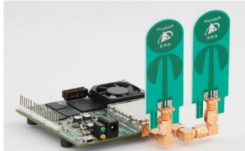
Fig 31: PulsON 410 MRM with both antennas connected
