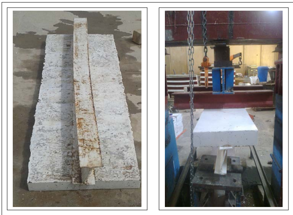
Figure 6: Beam CBEO2II at failure
