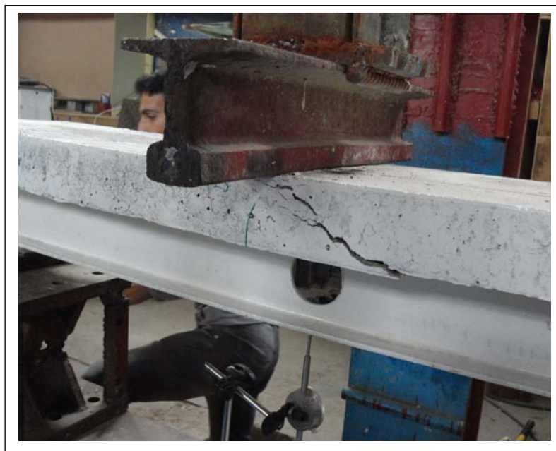
Figure 4: Beam CBO1 at failure
