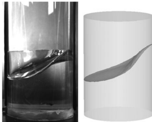
Figure 15. Interfaces of an aqueous solution of 98.5% glycerine at 125 rpm captured during an experiment (left) and its numerical counterpart (right). The shaking radius was 2.5 cm and the liquid height 10 cm.
