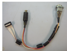
Figure 4.6. Wire that connects the DAS board with the RF downconverter
