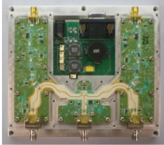
Figure 4.2. Real image of the Ka-band to L-band downconverter
