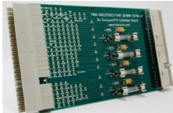
Figure 5.2. 3U Extender card used to provide power supply to the DAS board.
