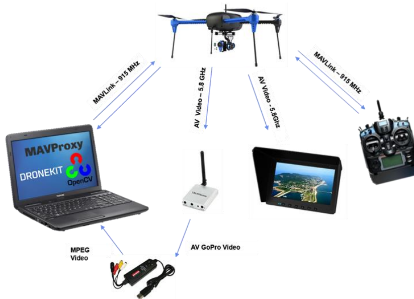
Figure 6 Ground target chasing system description
