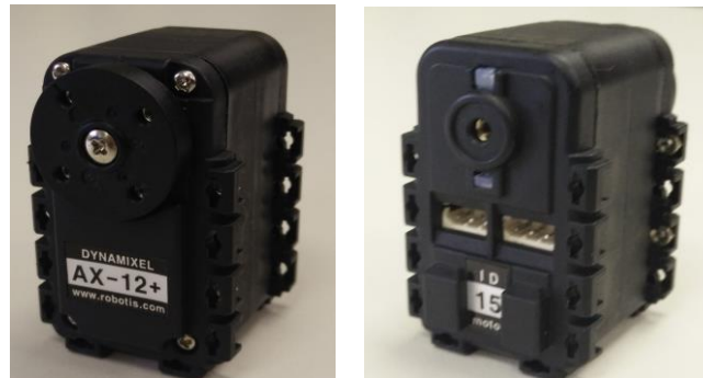
Fig. 3.3 Servomotors AX-12+ vista frontal i vista del darrere
