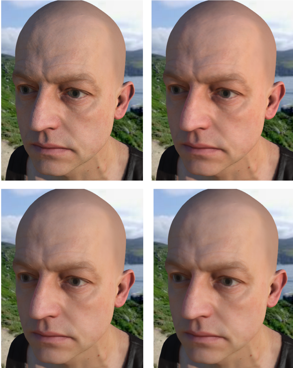
FIGURE 5.2: Methods comparison: original (top left), screen space sum of gaussians (top right), separable Artistic (bottom left), and pre-integrated kernel (bottom right).
