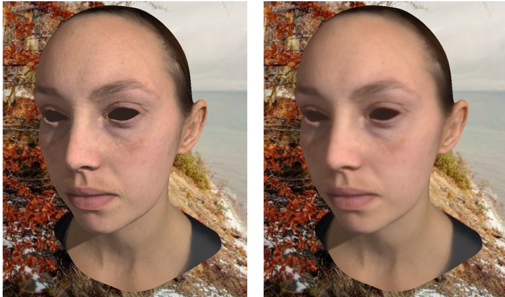
FIGURE 3.5: Comparison between two renders, the original render without subsurface scattering (left), and the one using the pre-integrated kernel subsurface scattering technique (right).
