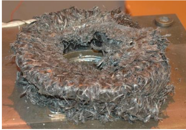
Figure 3: Picture of the splaying mode of energy dissipation
