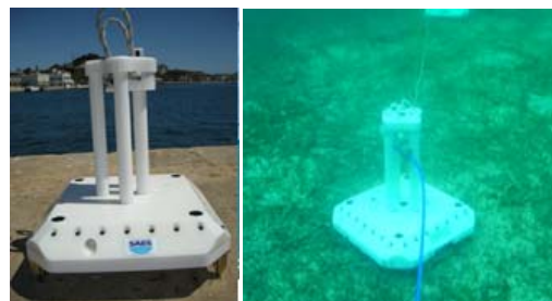
Fig. 2. Underwater Sensor Units (USU) of the Multi-Influence Range System, MIRS.
