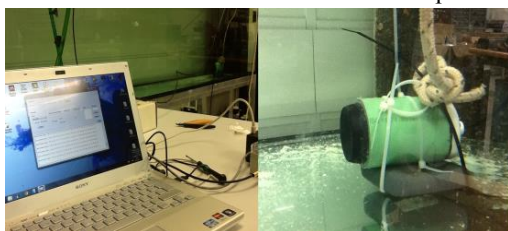
Fig. 2. Set up for testing in a UPV-lab the acoustic communications capabilities of the Alba-14
